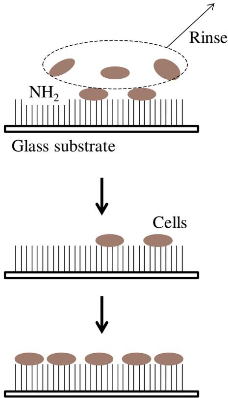
**Fig. 2:** Schematic view of the preparation procedure of a “diatom chip.” Cell suspension was placed as drop onto the surface of a functionalized glass slide. After a 1-h incubation period, unadsorbed cells were removed by rinsing. Thus, diatom cells were cultured on the functionalized glass surface.
