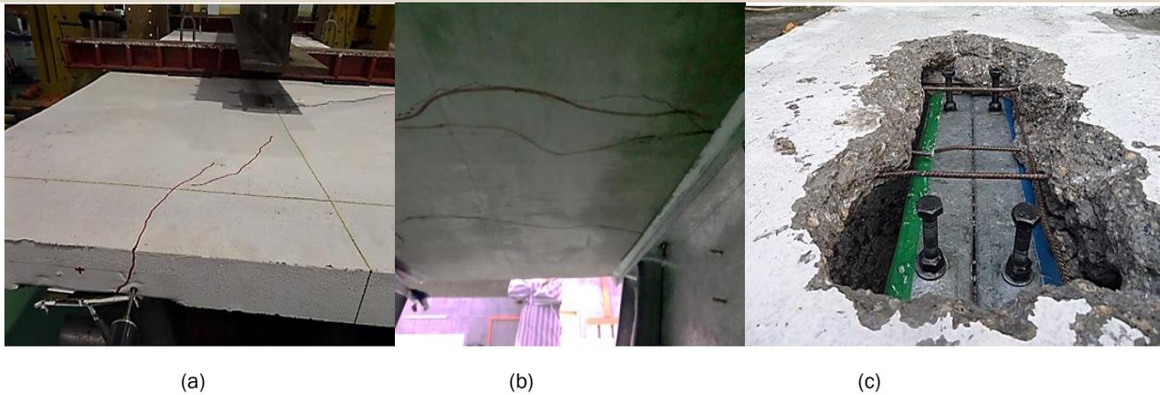
**Fig. 4:** (a) Concrete cracks on slab surface, (b) Transverse cracks beneath the slab, (c) Non-deformed shear connector.
