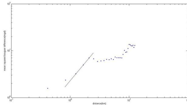
**Fig. 3:** Complete regression line of bouguer anomaly of the area with optimal density ( $2.8g/cm^3$ ) with fractal dimension (2.21)
