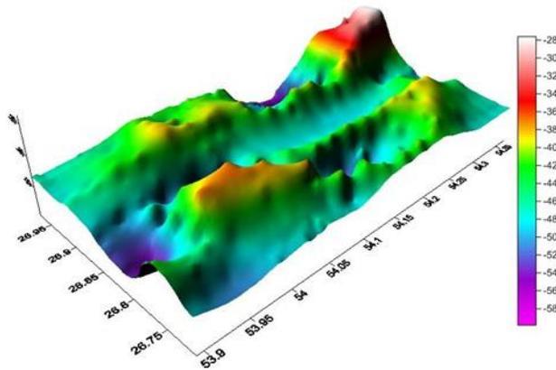
Fig. 1: Complete bouguer anomaly with density (2.5)g/cm<sup>3</sup>
