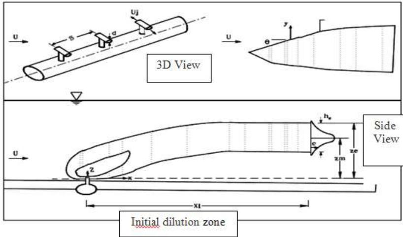
Fig. 2: Exit of effluent plume from diffuser into the sea with marine parameters [4].
