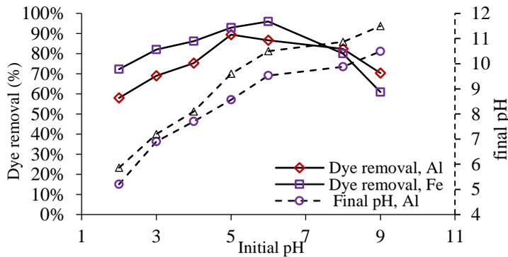
Fig. 1: Effect of pH on removal efficiency (time 80 min, 30 voltages, 5000 mg/l dye, 3000 μs/cm electrical conductivity).
