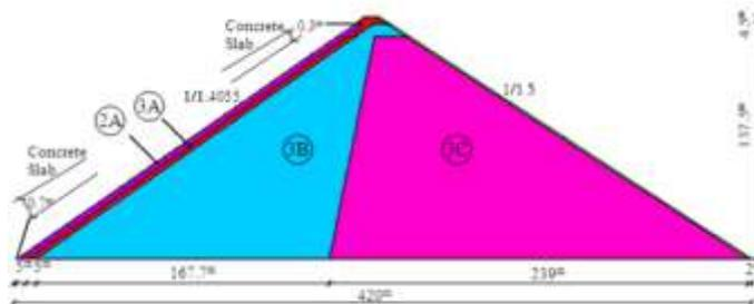
Figure 1. Two-dimensional cross-section of CRF dam [10]
