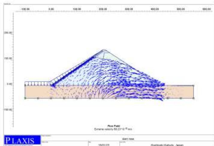
Diagram 11. The free surface flow in the dam body (Sakaria record)
