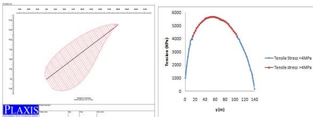
Diagram 4. The maximum axial, compressive and tensile stress rate (A) and maximum axial tensile stress (B) in the concrete face (Northridge record) in the empty tank case
