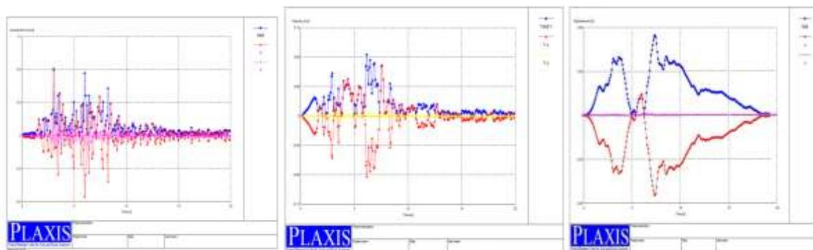
Diagram (3) Time history responses of acceleration (A), velocity (B) and displacement (C) of Northridge earthquake in the empty tank case
