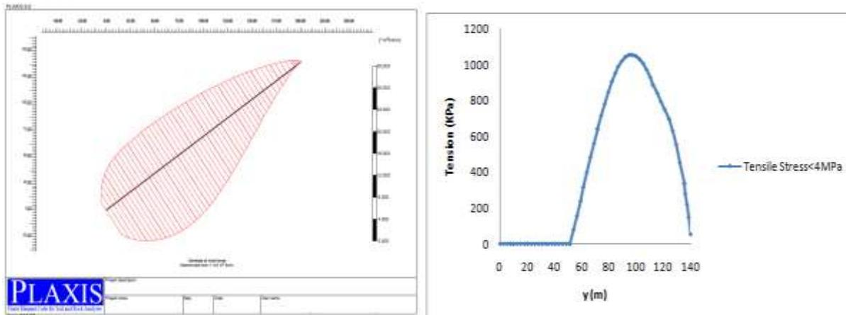
Diagram 6. The maximum axial, compressive and tensile stress rate (A) and maximum axial tensile stress (B) in the concrete face (Sakaria record) in the empty tank case
