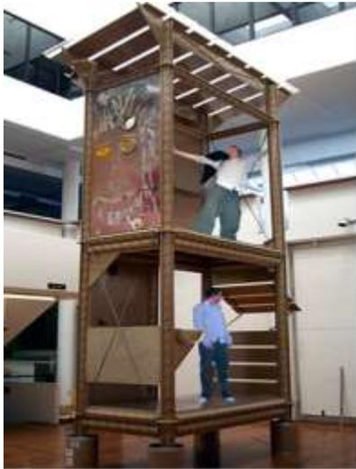
**Fig. 4:** The final structure made up of structural or non-structural paper components.
