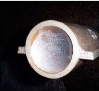
**Fig. 3:** Final cross section of structural paper component.
