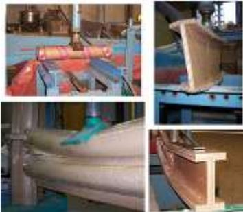
**Fig. 2:** Examining mechanical strength of structural paper components.
