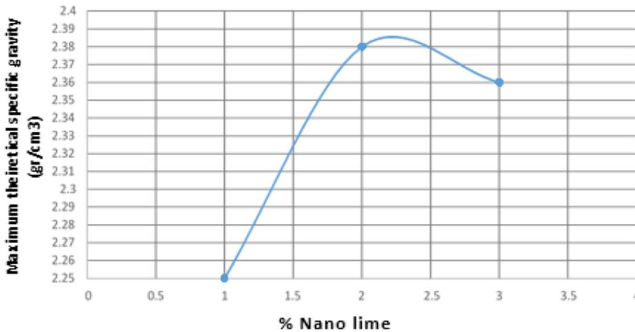
Fig. 9: Maximum theoretical specific gravity changes - Nano Lime.
