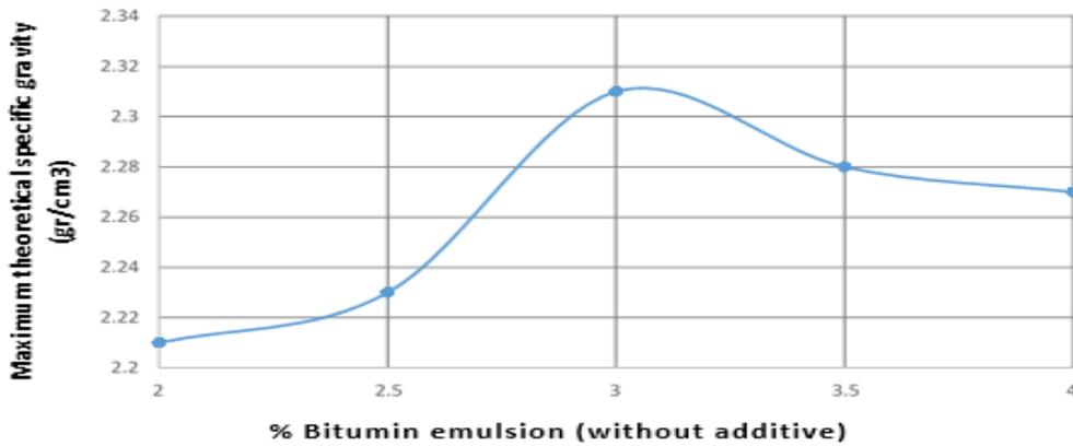
**Fig.3:** Maximum theoretical specific gravity changes - the percentage of bitumen emulsion (without additives).
