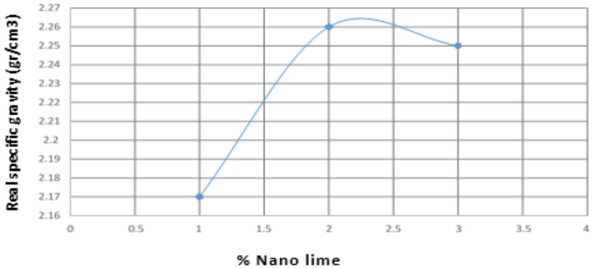
Fig. 8. Real specific gravity - Nano-lime percent.
