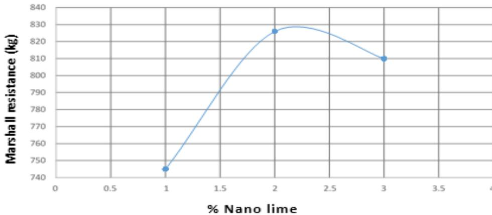
Fig.6: Marshall Resistance changes - the percentage of Nano Lime
