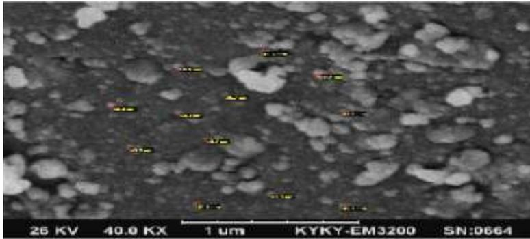
Fig. 5: SEM image of zirconium dioxide nanoparticle.
