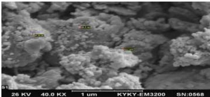
Fig. 6: SEM image of cellulose-zirconium dioxide nano composite.
