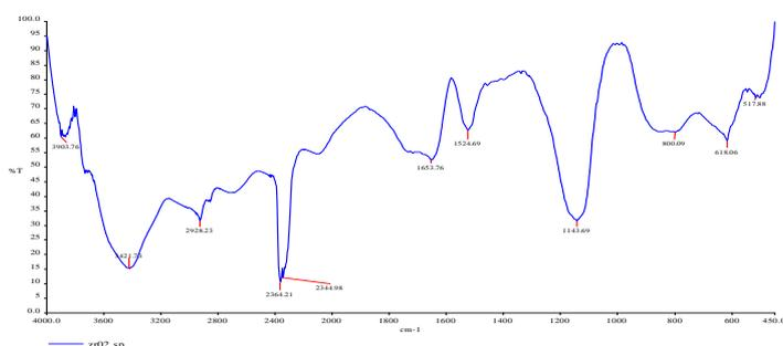
**Fig. 1:** FT-IR spectra of pure zirconium dioxide nanoparticle.
