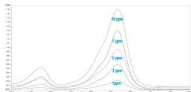
Fig. 7: UV-Vis spectra of MG solution (0-10 ppm).
