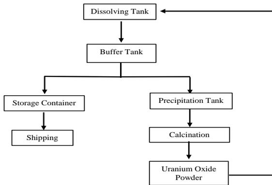
**Fig.1 Block Flow Diagram for the Purification Process at the JCO Reprocessing Plant [6]**
