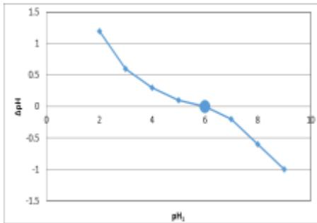
Fig. 6: Diagram of  $\Delta$ pH variations according to pH<sub>1</sub>.
