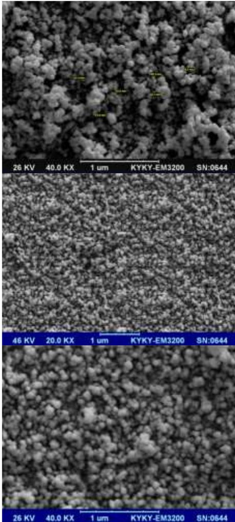
Fig. 3: SEM images of zinc titanium oxide nanoparticles.
