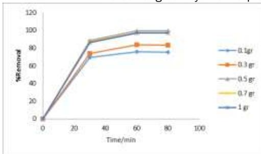
**Fig. 9:** Removal of malachite green on different contact time.
